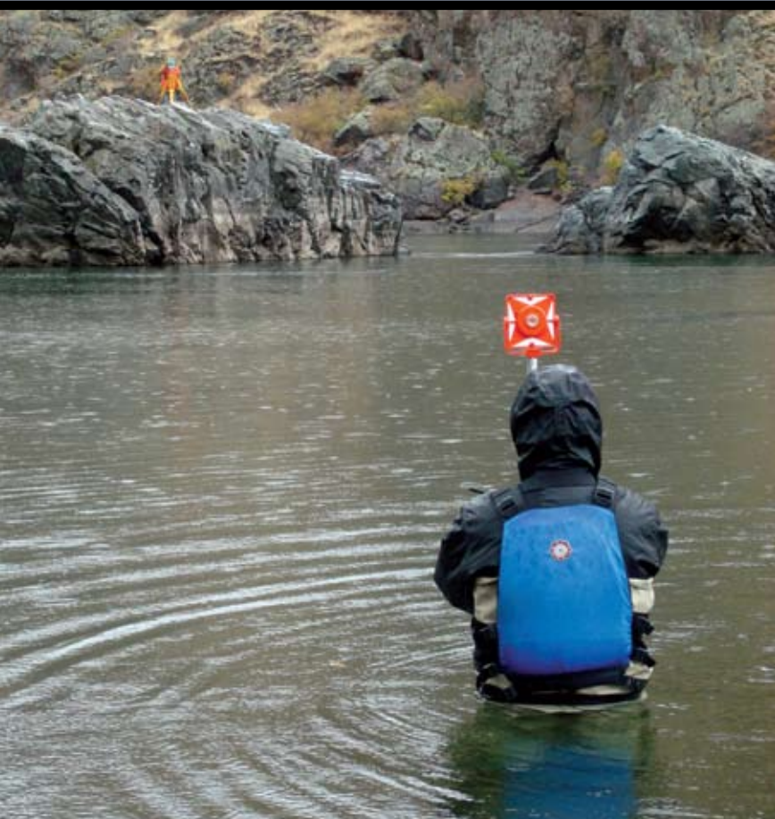
An Idaho Power hydrologist holds a level rod as a Glahe & Associates field technician collects sub-aquatic topographic transect data using a reflectorless total station from an isolated control point in the middle of the river.
