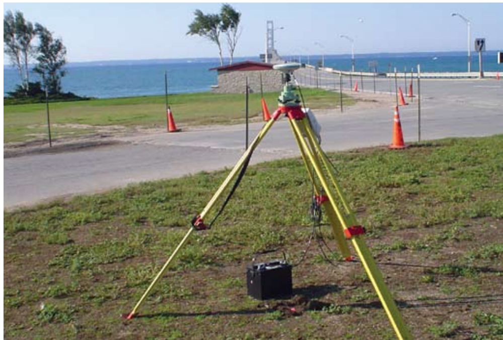
Two receivers on either side of the bridge served as static bases and logged many weeks of continuous one-second data using 1 gigabyte Compact Flash cards.
